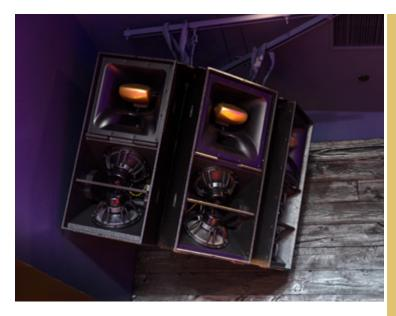
mong the products, the team utilized 12 of the XY-2E which allows the venue to build point-source arrays in a wide variety of configurations. The XY-2E maintains the favored X-phase system while enabling individual control of the 8-inch cone driver and 1-inch compression driver.
